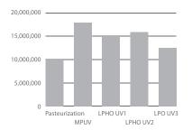
Figure 2. Net present worth for pasteurization and UV systems UV = ultraviolet MP = medium-pressure LPHO = low-pressure, high-output
